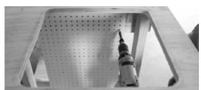
17 Attach the side and back pegboard panels (P and R) in the same manner, leaving the finished (white) sides facing the outside on the side panel and the inside on the back panel.
