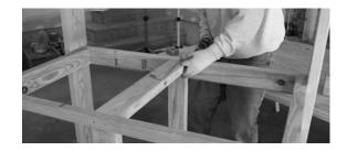
**07** Install bottom front stretcher (I) to front edge of both lower stretchers (F), keeping tops flush. Use glue and 2" screws.
