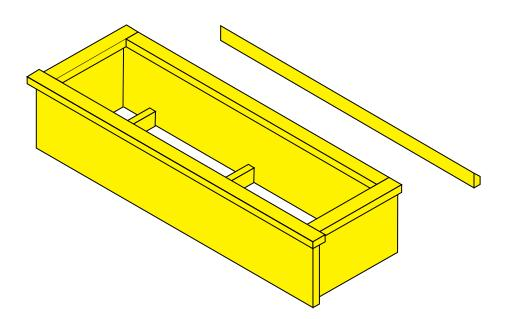
**TIP**: If using a hammer and finish nails to attach pieces, you will have to drill pilot holes so as not to split the wood. Set all nails below the surface with a nail set. These steps are unnecessary when using a finish nailer.
