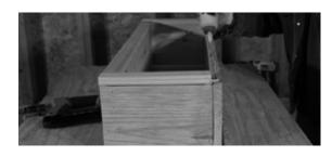
**09** Break all edges and touch up rough spots with sandpaper. Make sure all nail heads are set below the wood surface.
