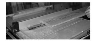
**02** For the cleats (I & J), which will be used to hang the box on your house, set your table saw's blade at 45° and rip the remaining 1 x 6 stock down the middle. Reset your saw blade to 90° and rip both pieces to 1 ½" wide.
