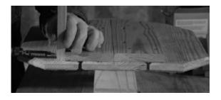
**10** Using the same techniques and order (two bottom pieces, then top, then the rest), attach the slats to the front (B/C/D) assembly.
