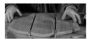
Once the glue has set on your inner support assemblies, rip them to 9" wide. Trim an equal amount from both sides, leaving the glue seam in the center of the panels. This will make centering the supports on the center panels and post much easier. Mark the radius according to the dimensions on the illustration, cut and sand smooth.
