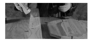
**08** Cut slats (E) and drill pilot holes 3/8" in from edge and centered along width.
