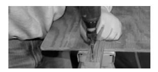
O9 Attach slats to back panel (D). Start with the bottom slats on both sides, then the top slat, and then fill in the rest of the slats with ¼" spacing. Drill pilot holes into edge of (D) to avoid splitting. This will leave an approximate ¾" space at the face of the slats (E) and a narrower space along the backside where they attach to part (D).
