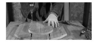
**07** Attach one finished (B/C/D) assembly to post with glue and 3" screws, with top of (B) centered 4" from top of post.
