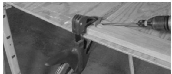
**05** Unclamp the piece and you have a very secure joint with fasteners that are invisible from the face.
