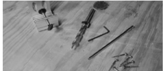
**02** Insert the drill bit until the collar stop rests on top and make sure the tip does not come in contact with the bottom of the jig (leave about 1/8" +). You may also mount the jig to your workspace, but this is optional.
